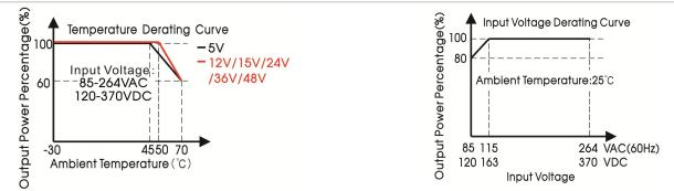
Note: 1. With an AC input voltage between 85-115 VAC and a DC input between 120-163 VDC the output power must be derated as per the temperature derating curves;
