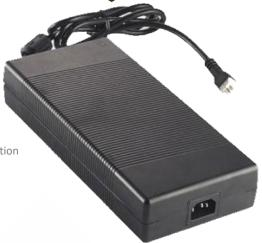
The Tiger Power range of switch mode power supplies feature a full comprehensive range of safety approvals for truly global requirements and meet latest level VI energy efficiency legislation. The TP1142 24vdc 300W model provides a reliable constant voltage output at up to 12.5 amps continuous, suitable for a wide range of applications.
