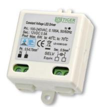
The Tiger Power range of LED drivers are highly reliable and meet latest safety and energy efficiency legislation. The TGR-12V-6W-B provides a 12vdc constant voltage output at up to 500mA (6W) suitable for a wide range of applications including LED strip lighting.
