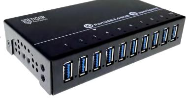
The Tiger Power range of industrial USB chargers are safety approved and highly reliable, meeting latest level VI energy efficiency legislation. The TGR-10P-USB model has 10 ports, allowing for an office or classroom to charge and sync their device at the same time via the 1 amp outputs. USB 3.0 spec for ultra fast data sync of up to 5Gbps. Suitable for a wide range of applications.
