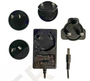
The Tiger Power range of switch mode power supplies feature full safety approvals to latest 62368-1 standards and also level VI energy efficiency requirements. The TP1128 5vdc 3A amp model provides a reliable constant voltage output at up to 15 Watts continuous, suitable for a wide range of applications.
