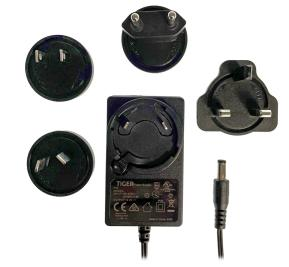
The Tiger Power range of switch mode power supplies feature full safety approvals to latest 62368-1 standards and also level VI energy efficiency requirements. The TP1001 12vdc 3A amp model provides a reliable constant voltage output at up to 36 Watts continuous, suitable for a wide range of applications.
