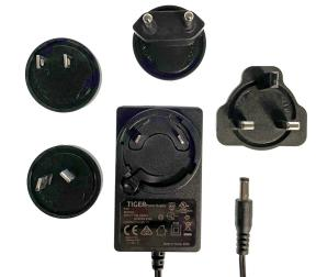
The Tiger Power range of switch mode power supplies feature full safety approvals to latest 62368-1 standards and also level VI energy efficiency requirements. The TP1127 12vdc 2A amp model provides a reliable constant voltage output at up to 24 Watts continuous, suitable for a wide range of applications.
