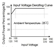
Note: ① With an AC input between 85-100VAC and a DC input between 120-140VDC, the output power must be derated as per temperature derating curves;
